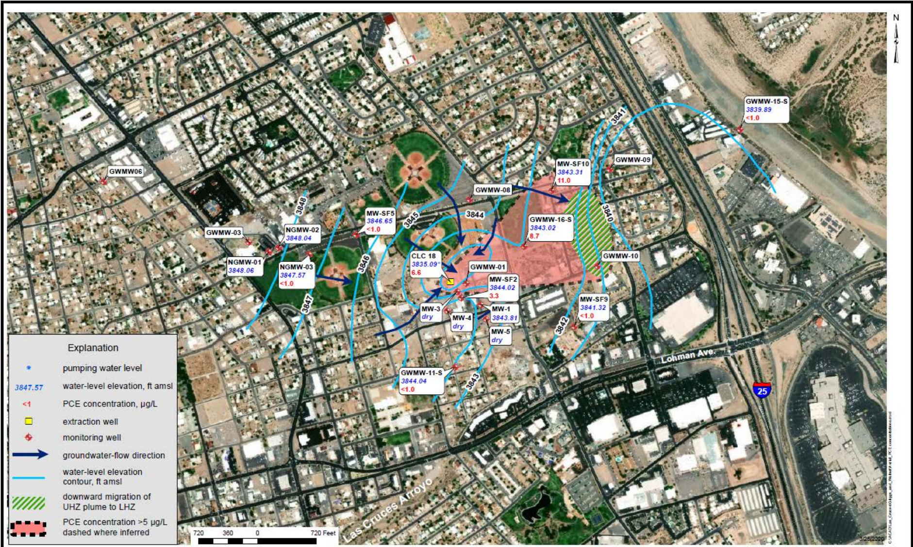
Figure 12 – Upper Hydrogeologic Zone Ground Water Elevation Contours and PCE Concentrations, December 2019 (JSAI, 2020)
